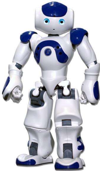
Figure 1: The Nao humanoid robot. The Nao is approximately 58cm high, with 25 degrees of freedom. Picture source: http://www.aldebaran-robotics.com/
